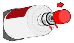
Insert new cartridge and turn until it locates. Install with a quarter-turn to the right until cartridge comes to a complete stop (Inlet water will automatically turn on).
