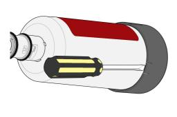
4. With one tab loosened, pull the filter cap off the old cartridge.
