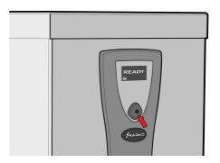
2. Grip cartridge and rotate a quarter-turn to the left and pull forward. CAUTION: A small amount of water will drain from the head
